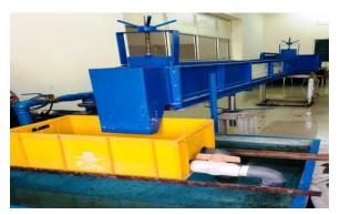
Fig.2 Tilting Flume
