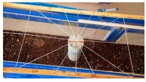
Fig.1 Arrangement of Pier in Tilting Flume
